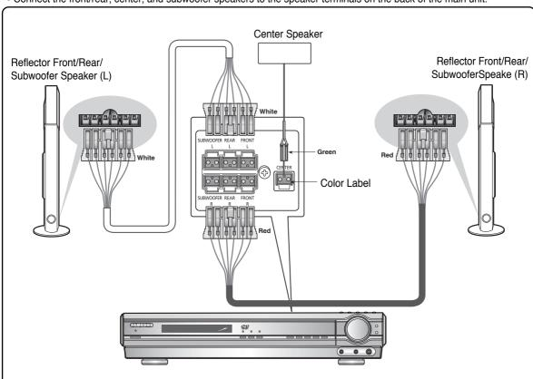
• Connect the front/rear, center, and subwoofer speakers to the speaker terminals on the back of the main unit.
